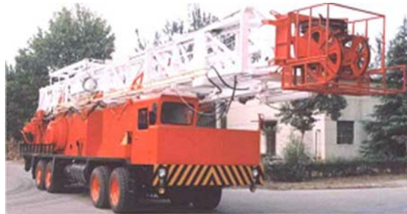
Truck Mounted Drilling Rig
